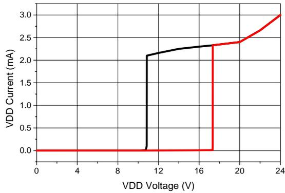
VDD Operation Current vs Load
